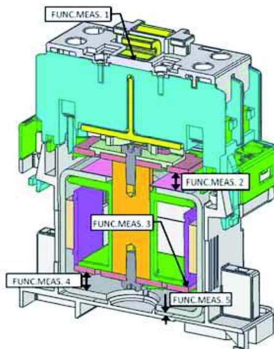
Fig. 1 - Contactor section highlighting the 5 functioning measurements
