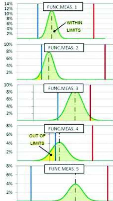
Fig. 2 - Distributions of functioning measurements in the virtual production
